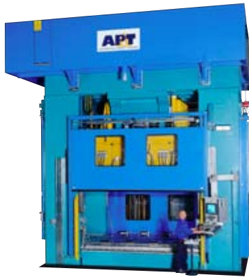
HF Short stroke press Forces up to 100,000 kN Bed up to 3,600 x 2,700 mm Tie rod design Prism guiding of slide
