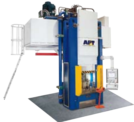
HMD A hydroforming press with an oil supported diaphragm. Forming pressure 35/70/100 MPa Blank diameter \varnothing 380/635/810 mm Press frame force 9,200 - 40,000 kN
