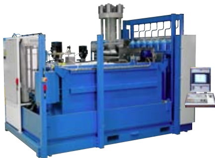
HPS Retrofit Water and hydraulic high pressure system with HNC control for retrofit. Includes functions like quick-fill pump, pre-form pump, pressure intensifier, tool axes and on/off valves.
